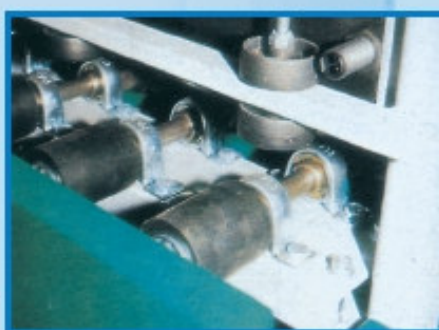
Distanza minima tra i rulli di trasporto, rulli movimentati singolarmente, finecorsa con fotocellula. Small distance between transportation rolls, every single roll driven separately, end-stop by photocell.
