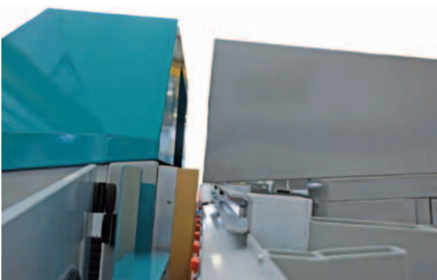
All M-RX 130 machines are open top and therefore also suitable for bigger sheets (processing up to 1300mm)
