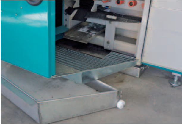
Water tank in two pieces for easy dismantling and cleaning
