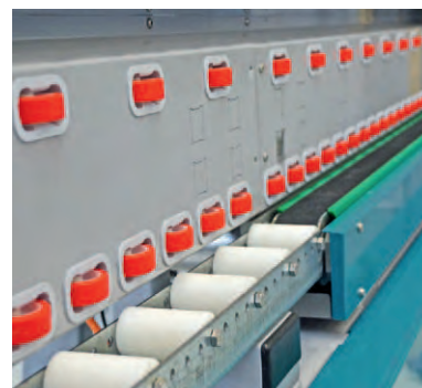
Extension modules with rollers or with precision belts
