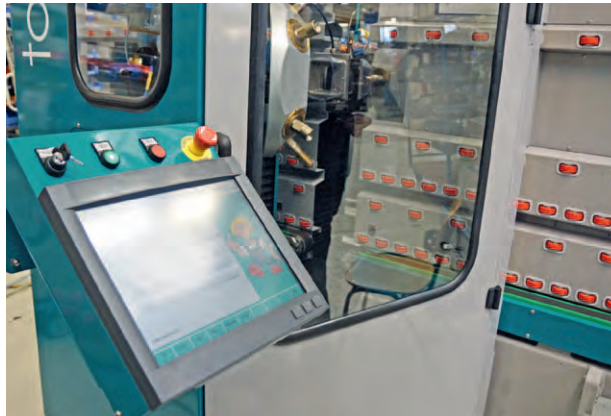
operator panel, foldaway, for optimal view
